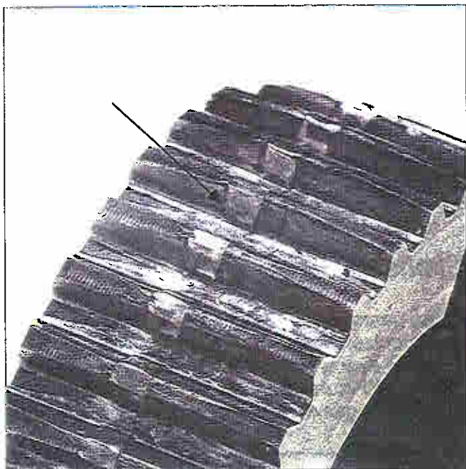
Figure 20—Worn gear locks on the clutch gear can lead to gear jumping.
