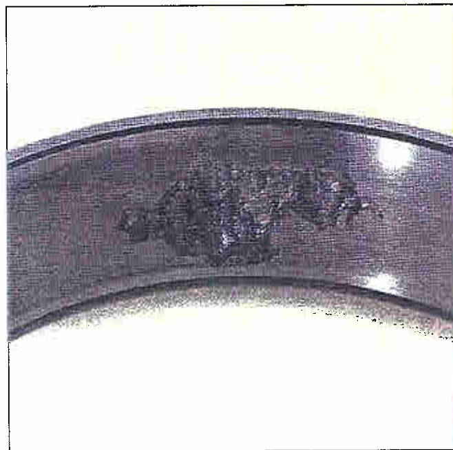
Figure 10—Offset spalling is caused by misalignment.
